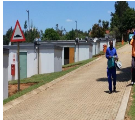
Figure 3-8: Kerbs forming a channel along the segmented block paving
